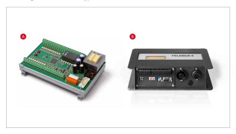
With the universal interface solution, weld process controllers can be connected with all industrial robot types. Users basically have two options for connecting robots with weld process controllers: The connection can be realized with the interface UNI 5 or by integrating into a given field bus environment with a field bus solution.
